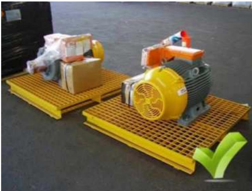
A very well packaged consignment, alternators have been bolted to the metal pallet and the cartons metal strapped. Can be easily loaded and unloaded.
