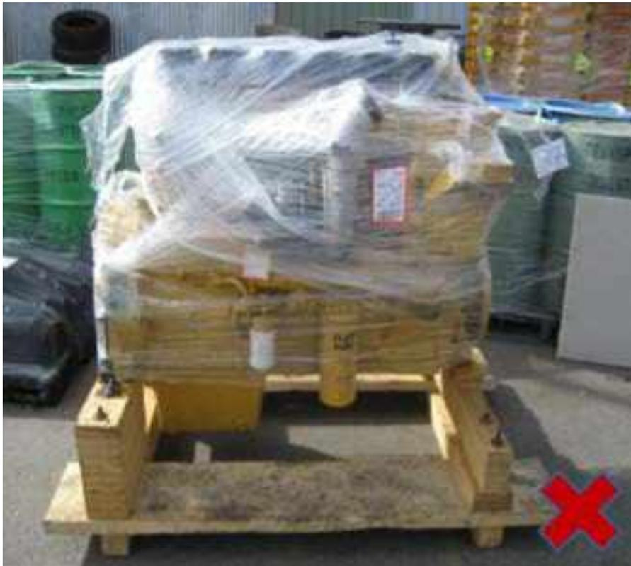
These heavy roller pins have had restraints applied over the pallet top slats and not the pallet under bearers.
