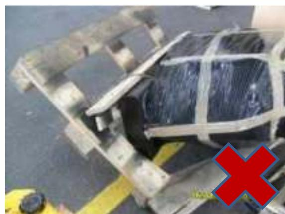
The selected pallet Safe Work Load (SWL) must be capable of successfully supporting the loaded weight. When selecting pallets, consideration should be given for item centre of gravity, height and distribution on pallet.
