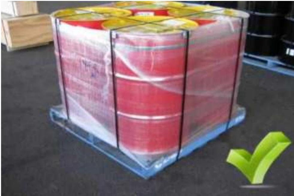
These drums are well packed, the banding prevents movement during transit and handling. Further drum packaging techniques are shown in Section 21.1.
