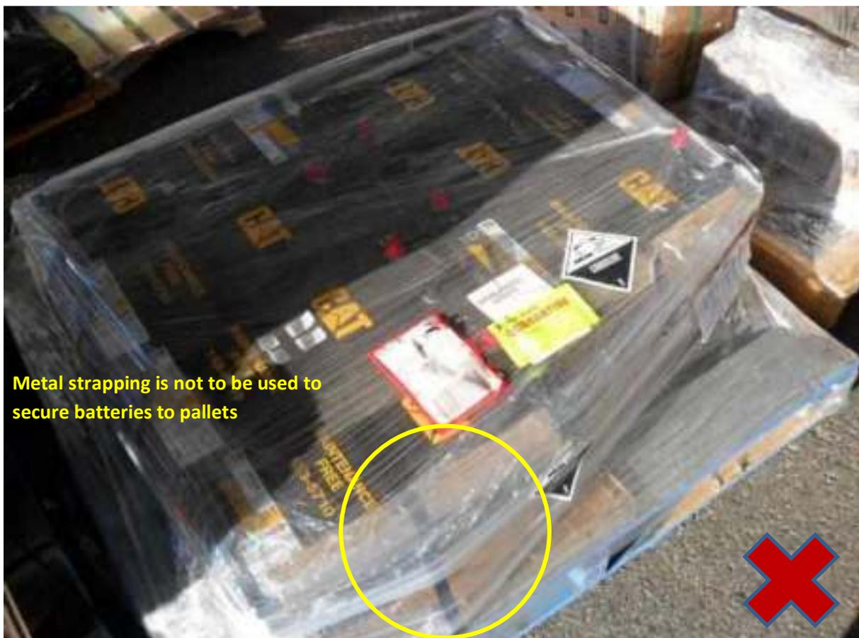
Strapping with plastic strapping only, should be sufficiently applied to prevent movement and possible dislodgement from pallet.
