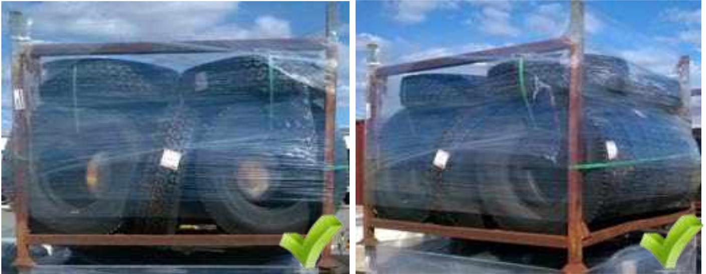
Examples of tyres strapped to pallets to prevent movement:
