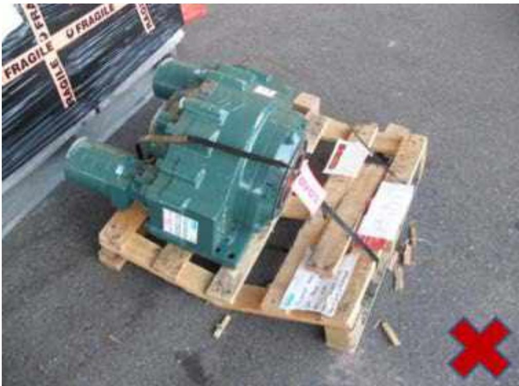
Soft pine skids do not effectively hold up for transport. All remanufacture wood products for crates, pallets and skids should be scrutinised prior to submission of freight.
