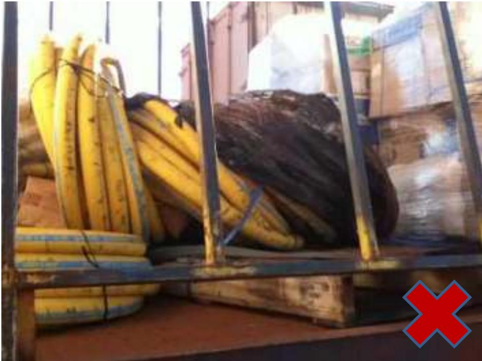
Hoses should be banded together with the use of either metal or plastic banding and restrained under the pallet bearers to ensure safe transport.
