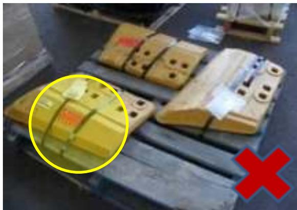
Restraint applied over top of freight allows heavy item to slide or walk from pallet
