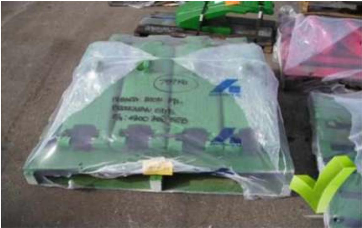
A well packaged consignment on a good sturdy pallet. Metal banding is under the pallet under bearers and goods are covered in clear plastic for further protection.
