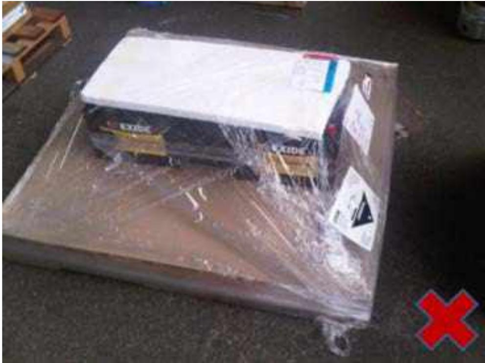
**Note:** Metal strapping is not to be used for securing batteries to pallets due to the potential of energising the battery if in contact with terminals.
