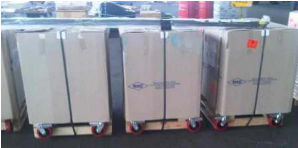
The above example highlights how to effectively limit movement from items supplied on wheels. These items must be stabilised for transport and the use of pallets underneath loads, with applied straps under the under bearers, is an example on how to limit movement for safe transport.
