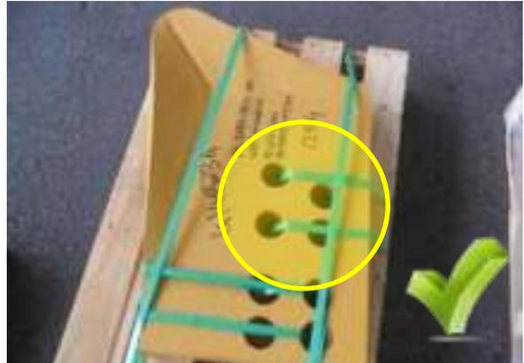
Preference is to have restraint through item keyholes to provide additional restraint
