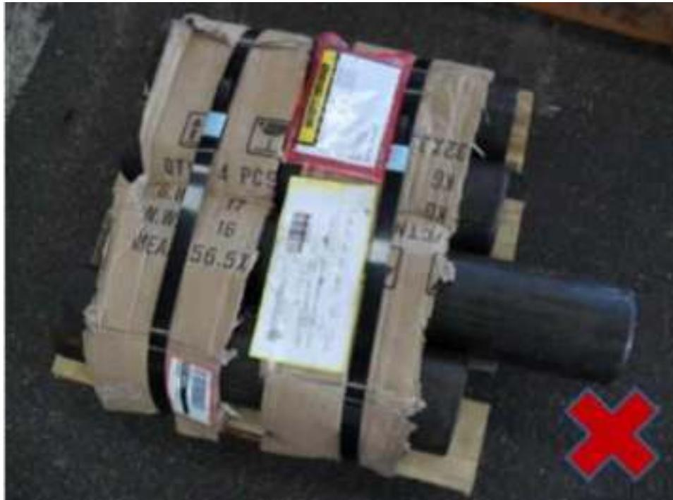
Item below is too heavy for the supplied skid and has collapsed under the weight of the item.
