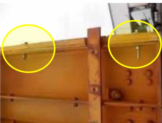
It is a requirement that all pulleys for Rio Tinto be provided in metal transport frames. One time/wooden frames are not deemed acceptable by Rio Tinto for the transport and safe handling of these cylindrical items.
