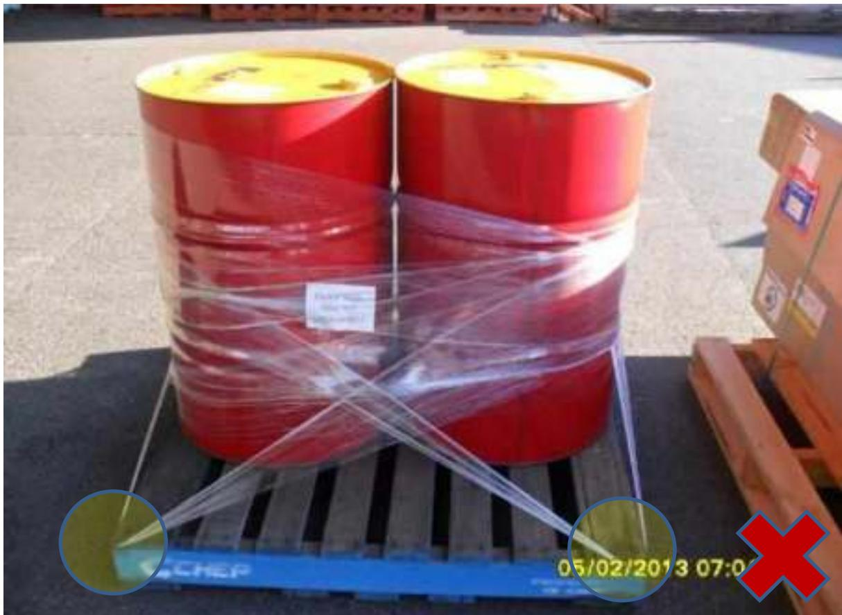
Plastic shrink wrap lifts the top slats and voids restraint.
