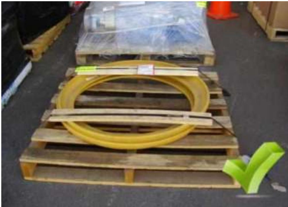
These drill rods are suitably packed for transport and handling.
