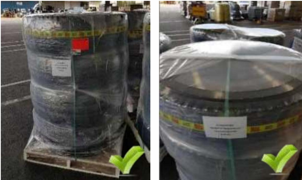
Alternatively, if unable to heat shrink the column of tyres, then the tyres must be plastic wrapped then strapped as displayed in the below image.
