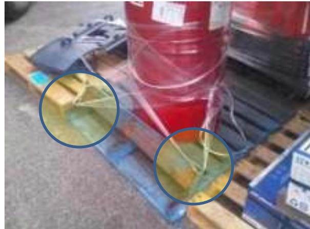
Applying straps/restraint over top slats without loaded weight lifts the slat, voiding the restraint.
