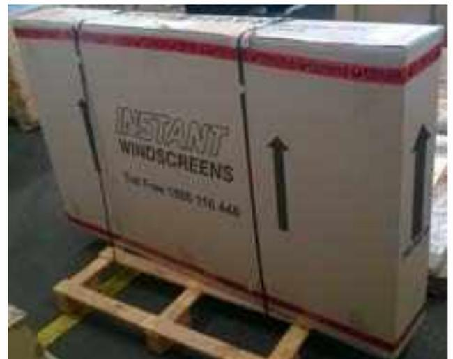
The use of plastic carton protectors will allow further tension on the restraint to be applied and ensure windscreens are restrained in the upright position. The image below depicts how these protectors are applied.
