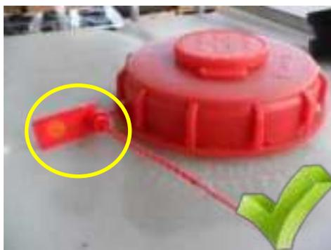
Outlet valves on IBCs must have secondary containment e.g. camlock cap or plug, screw caps.
