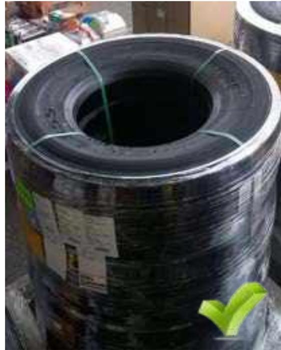
Tyres can also be strapped to pallets to prevent movement as below. Four (4) straps are required on a vertically stacked pallet with the straps running through the middle of the stack.
