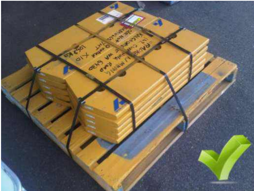
Heavy rolls effectively strapped under pallet bearers.
