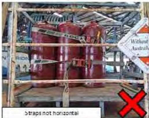
Gas cylinder without appropriate contact with adjacent cylinders
