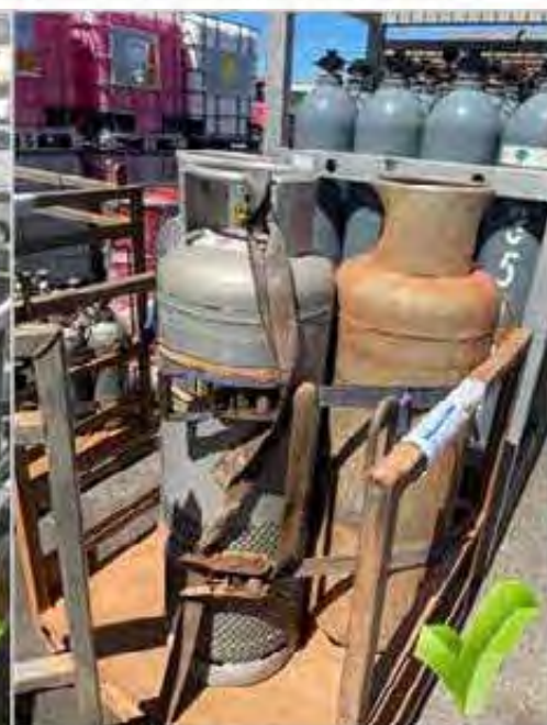
Load straps anchored close to cylinders in partly filled stillage
