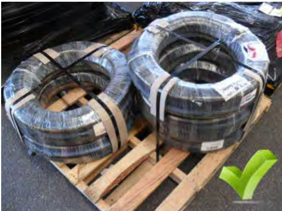
Hoses supplied on sturdy oversize pallet, suitably strapped with ends protected with plastic wrap.
